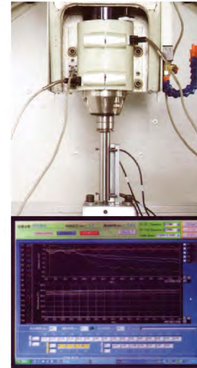
SPINDLE DYNAMIC BALANCE TESTING After machine assembly, the spindle is re-balanced to ensure smooth operation.
