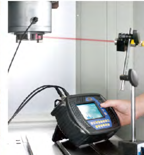
SPINDLE THERMAL GROWTH TESTING Each spindle is tested through the complete speed range and thermal growth is measured to ensure the spindle is within normal values.
