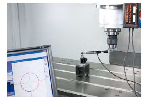
BALL BAR TESTING Every machine is put through a Dynamic Ballbar test to test circularity and reversal spike errors.
