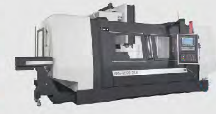
▲ 2590-2LB • Travel : X2500 Y1000 Z1000 mm • Table : L2600 × W1000 mm
