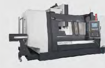
▲ 2090-2LB • Travel : X2000 Y1000 Z1000 mm • Table : L2150 × W1000 mm
