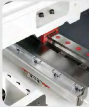
HEIDENHAIN Linear Scale
